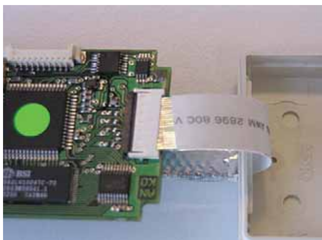
Figure 9 : Flexi cable misplacement.
