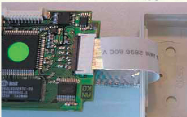
Figure A1 Flexi cable misplacement
