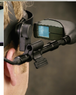
Figure 41: The monocular optical see-through display of the Mobile AR system
