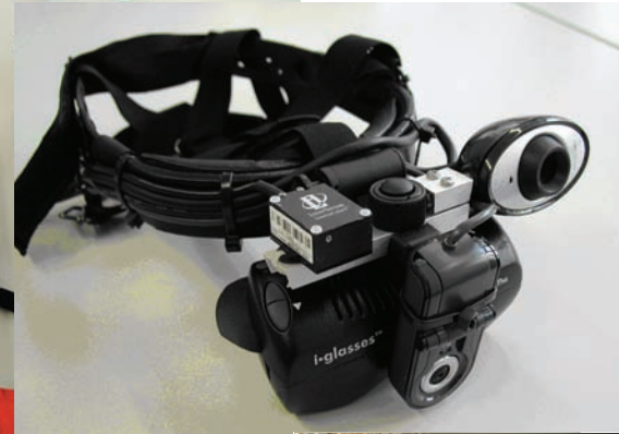
Figure 40: The full AR system :backpack with laptop, Headset with video see-through display and tracking hardware, and wireless mouse
